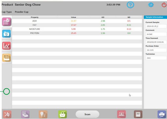
Versatile results display with warning and action displays for outlier and product limits
