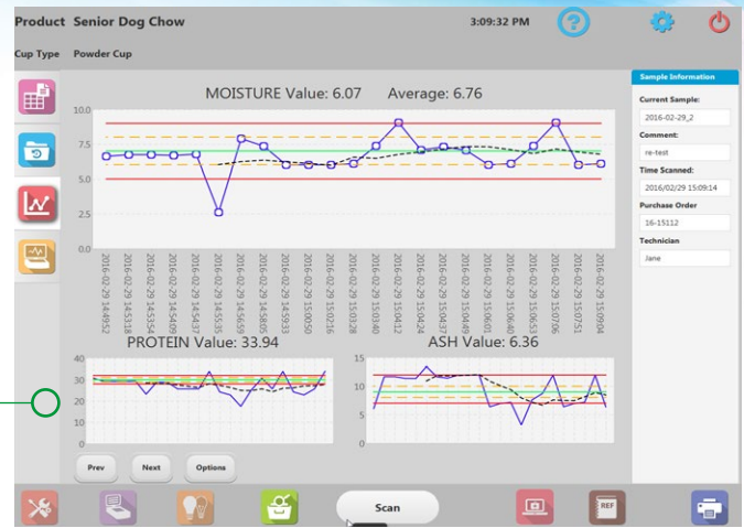
Configurable SPC view displays control charts for three constituents enabling immediate process control
